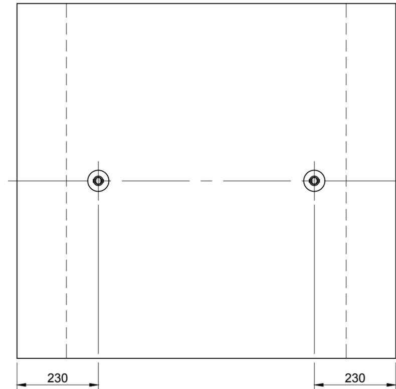
Recess Socket for M20 Nailing Plate.
