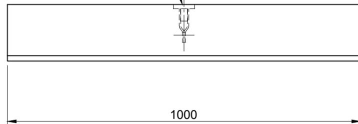
M20 Flat End Lifting Socket
